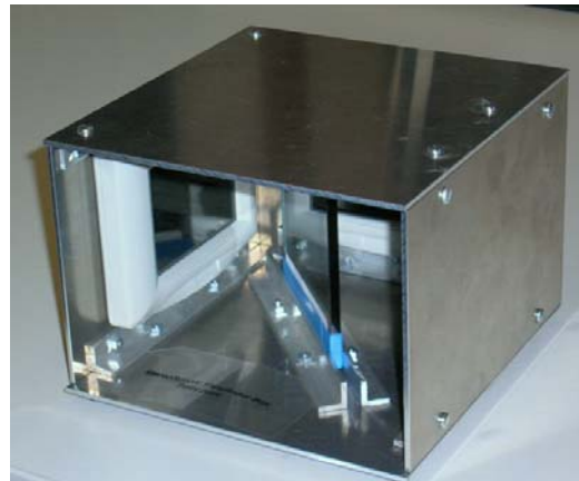
Image 6: Exterior of Stereoscopic Cube Viewfinder
